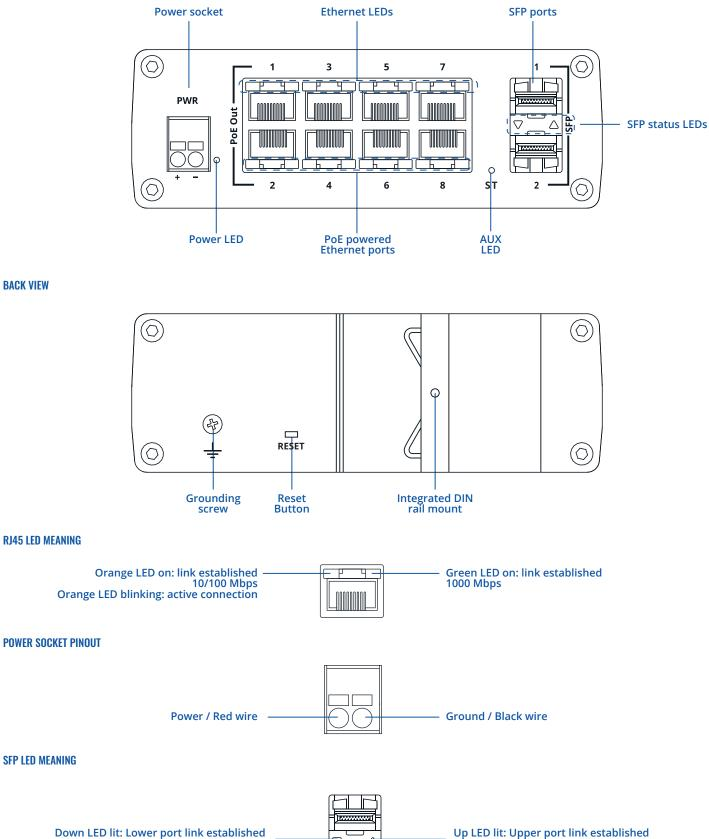
Down LED blinking: Lower port active traffic
