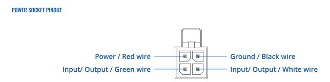
I/O (PIN 3 and 4): Configurable digital Input/Output pins. Open collector output, max output 30 V, 300 mA or Digital input where 0-6 V detected as logic low and 8-30 V – logic high
