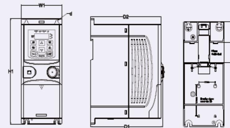
Rail mounting of inverters of 1PH 230V/3PH 400V ( $\leq 2.2\text{kW}$ ) and 3PH 230V ( $\leq 0.75\text{kW}$ )
