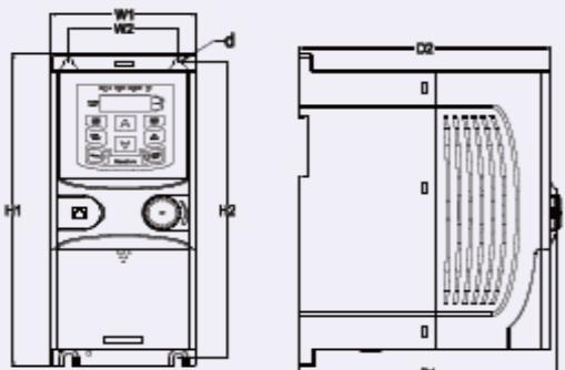
Wall mounting of 0.75~2.2kW inverters
