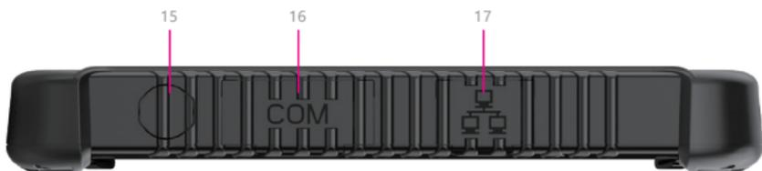
15.**Avigation interface:** Connect electrical wiring interface(need custom-made, standard configuration machine without the interface).
