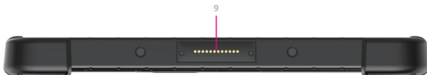
9. **Pogo pin**: connect docking , expand USB interface and network port / charging interface.
