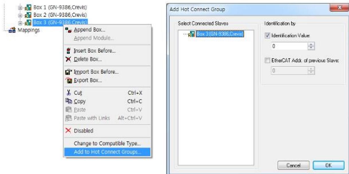
3. Hot connection group set up is completed, run the Reload I/O device(F4).
