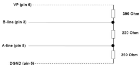
In order to minimize cable reflections and ensure a defined noise level on the data lines, the data transfer cable must be terminated at both ends with a terminating resistor combination as follows.
