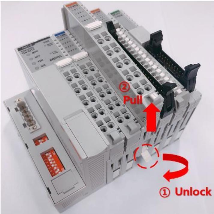
As above figure in order to safeguard the FnIO module from jamming, it should be fixed onto the DIN rail with locking level. To do so, fold on the upper of the locking lever. To pull out the FnIO module, unfold the locking lever as below figure.
